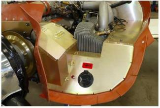
Figure 2 - SR22/SR22T Shore power plug located in left front engine baffle. Plug for the SR20 (not shown), is located in same area on horizontal surface of baffle.
